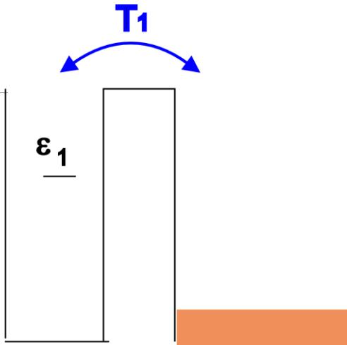
$$\hat{H} = \varepsilon_1 c_1^+ c_1 + \sum_k \varepsilon_k c_k^+ c_k + T_1 \sum_k (c_k^+ c_1 + c_1^+ c_k)$$
